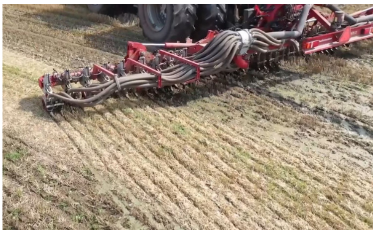
Low Disturbance Manure Injection
